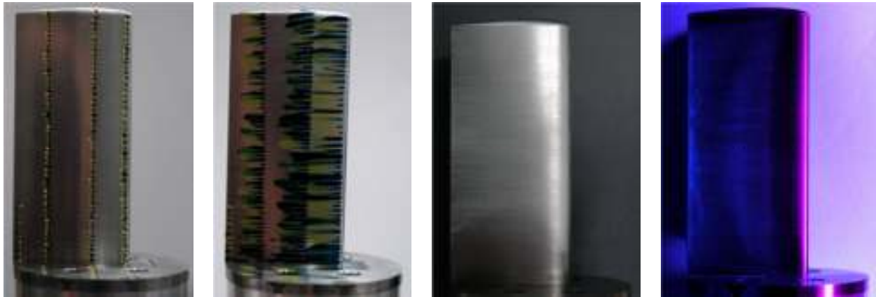
Figure 6. Images of surface oil flow visualization techniques with regular and fluorescent mixtures.
